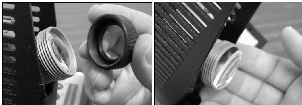
Remove retaining ring to access lens
