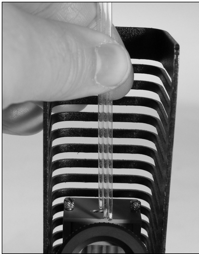
Loading capillaries into DigiMelt.
